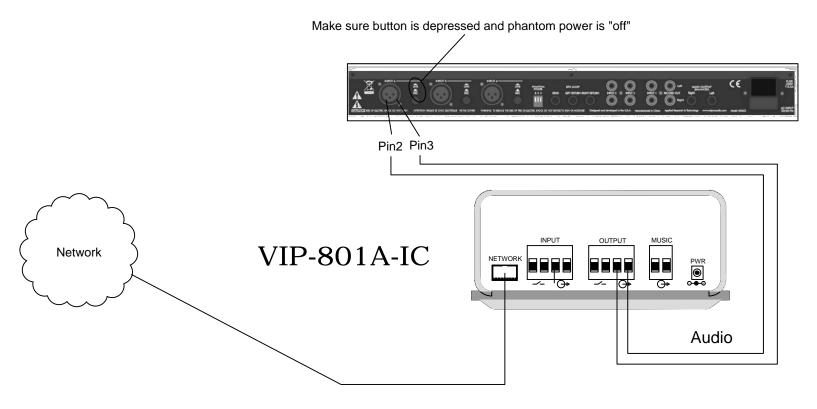
Within the VIP-102B Software, set the VIP-801A Channel volume slider to -15 to start. Adjustments may be made after testing.
